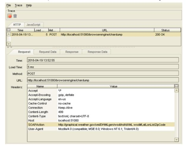
Copy the value of the **SOAPAction** header, switch to the updated robot and paste it to the property called **SOAP Action**. To copy the value, double-click the header in the list and copy its value from the **Show HTTP Header** dialog box.
